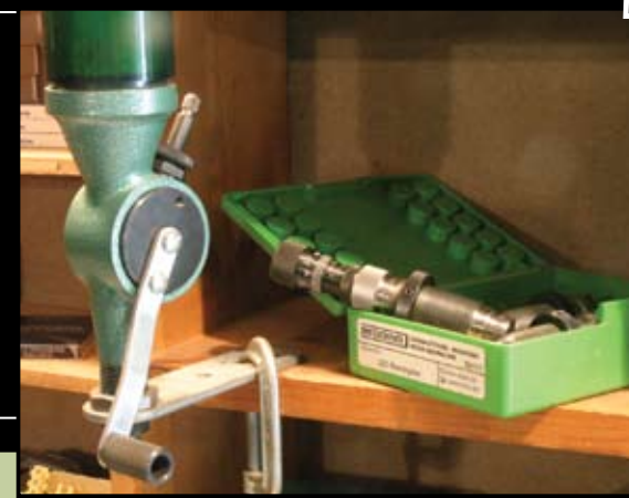
Two useful tools for producing lots of AR hunting ammunition are the powder measure and a precise bullet-seating die like this Redding Competition die.
